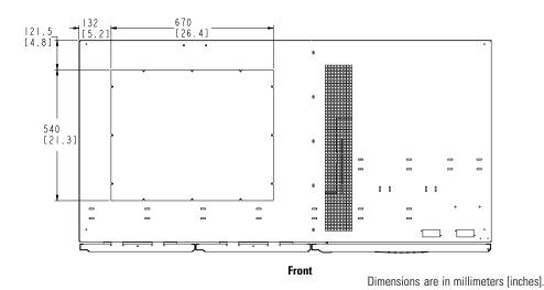
Figure 3-5. ISBM Section Dimensions (Top View)
